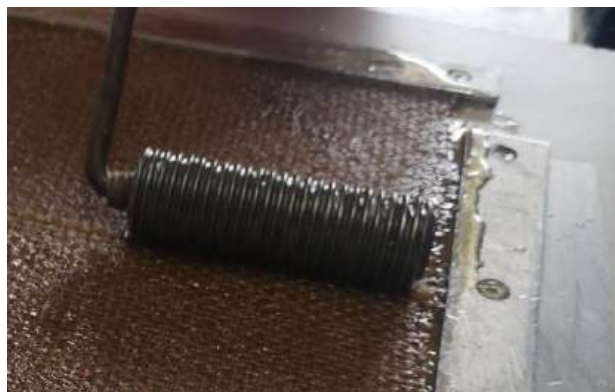
Figure 1: Hemp resin treated for air bubbles.
