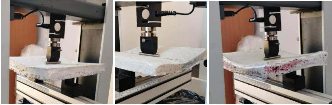
Figure 1: Plate samples during testing (a- plaster, b- cement, c- hemp-based)
