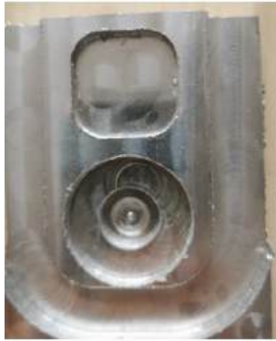
Figure 2: Machining at cutting speed of 500mm/min
