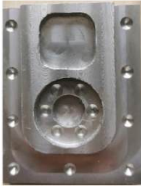
Figure 4: Machining at cutting speed of 150mm/min
