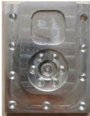
Figure 3: Machining at cutting speed of 500mm/min
