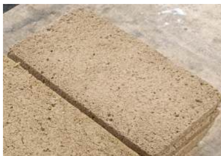
Figure 1: Composites made of recycled cardboard.
