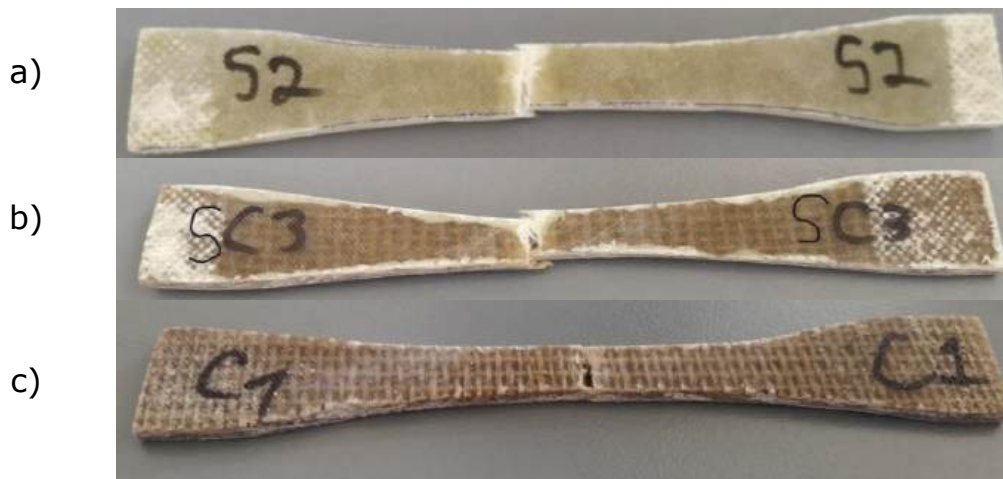
Figure 5: a) Test specimen Fiber glass after testing; b) Test specimen Fiber glass + Hemp after testing; c) Test specimen Hemp roving after testing.
