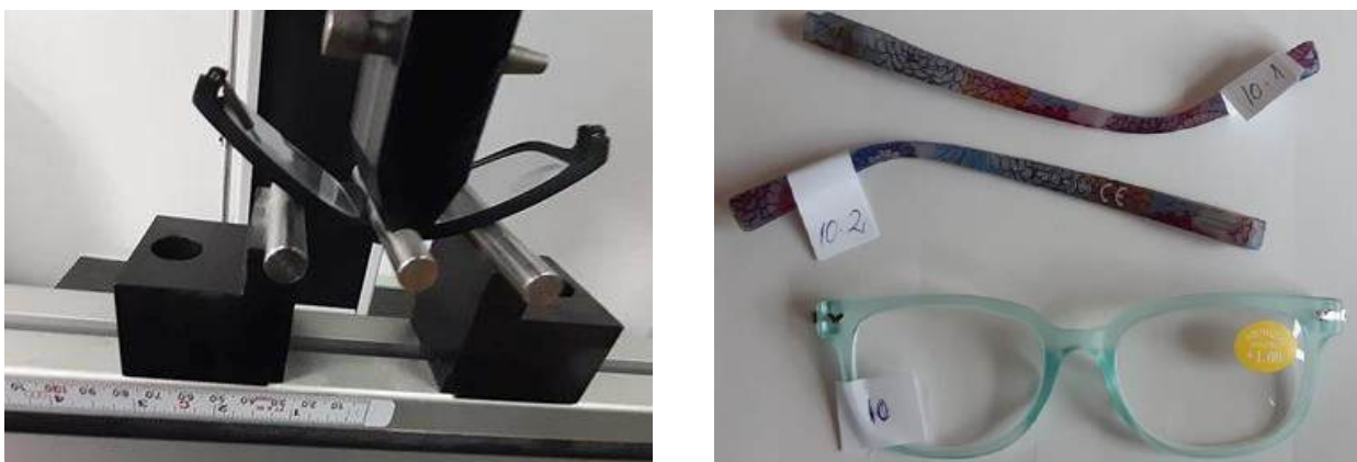
Figure 1: Glasses frames and arms subjected to bending test
