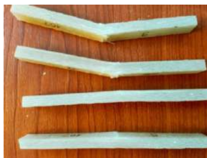
Figure 2. Composite material sample after bending stress
